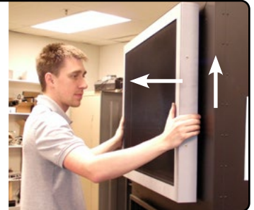
Figure 6.e Lifting screen frame up and out.
