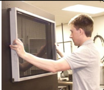
Figure 6.a Removing the screen
