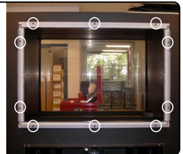
Figure 6.f Removing screws that secure screen.
