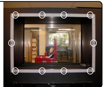
Figure 6.g Removing screws that secure screen.
