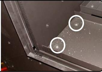
Figure 4.b Removing screws that secure media tray
