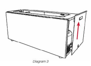
4. Remove 3 screws in locations shown below to remove side panel. Note: Coffee height table requires removal of only 2 screws (no middle
