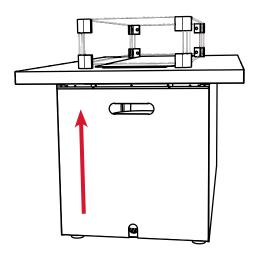
2. Loosen butterfly bolt to allow LP tank to be seated on the holder.
