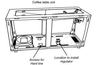
12. Install regulator bracket onto unit base with 2 screws. Connect flex line to regulator—position regulator onto bracket.
