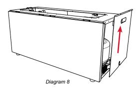
10. Remove 2 screws in locations shown below to remove side panel.
