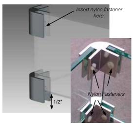
7. Place assembled glass surround/windshield on table top - ensure glass is centered on the table top. Once in correct position, lift up one end, apply double sided tape that has been cut to size, to the bottom of the brackets. Repeat process on other end. Press down firmly from to secure glass surround/windshield in position. Use care not to scratch surfaces.
