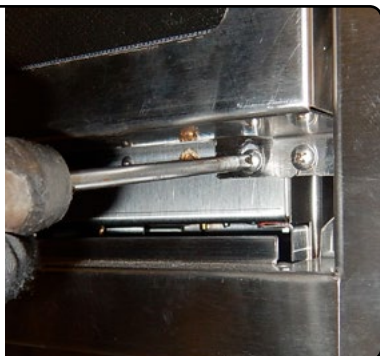
Figure 59 Removing the right side screw
