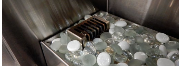
Figure 66 DO NOT place ANY firestones on top of the pilot cover).
