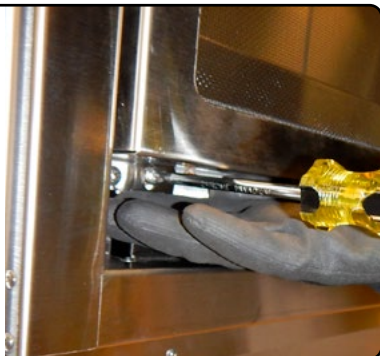
Figure 58 Removing the left side screw
