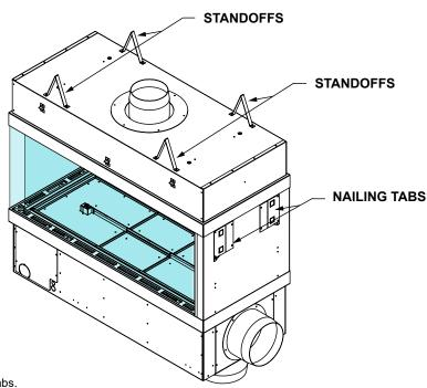
**Figure 4A.3** Placement of the standoffs and nailing tabs.
