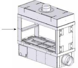
Install the threaded rods in the appropriate locations for A, B & C as noted below in D. THREADED ROS.
