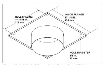
Figure 8D.2 10 Inch Chimney Collar Dimensions (RS14)
