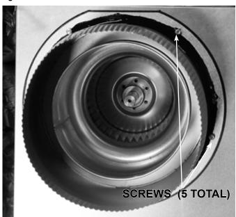
Figure 8F.4 Base Plate Fastened to Intake
