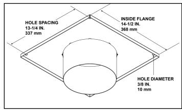
Figure 8D.1 8 Inch Chimney Collar Dimensions (RS12)
