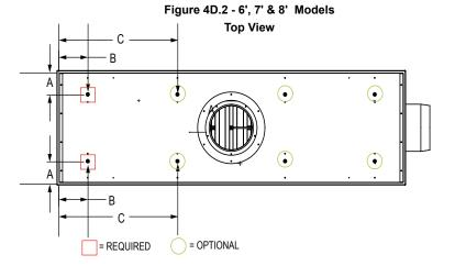
The hood shall be supported at specific locations using 1/4-20 UNC threaded rods.
