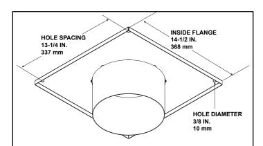
Figure 8D.1 8 Inch Chimney Collar Dimensions (RS12)
