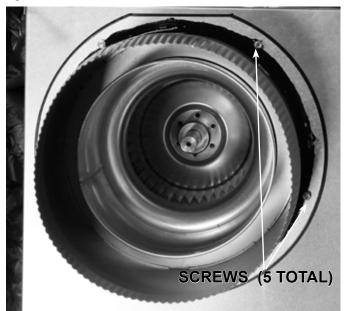
Figure 8F.4 Base Plate Fastened to Intake
