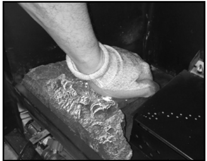
Figure 11.1 Press Left Hearth Firmly Into Place
