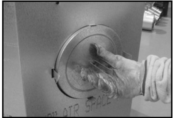
Figure 6.10 (Generic Fireplace Shown) Fold the center parts of the retaining band out and use to remove the seal cap.
